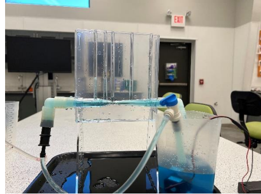
Figure 1. a) Hydraulic loss (left) and b) Venturi (right) set up
