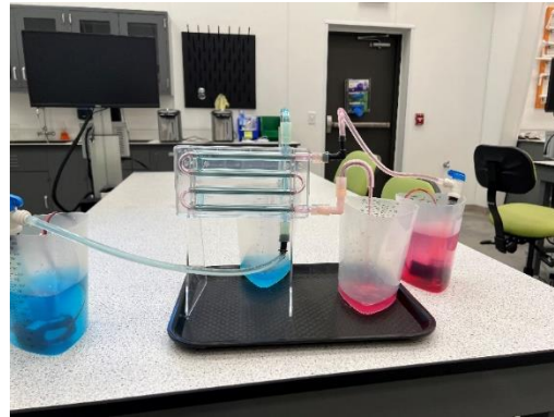
Figure 2. Double pipe set up
