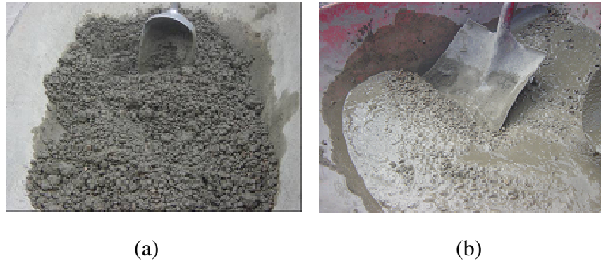
Figure 9. Comparison Between (a) 0.45 and (b) 0.60 W/C Mixtures
