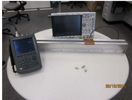
Figure 4. Test setup for slotted line experiment.
