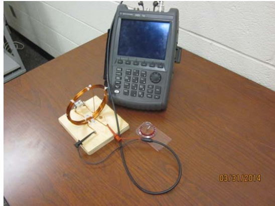
Figure 3. Loop antenna to direction find on frequencies below 2 MHz.
