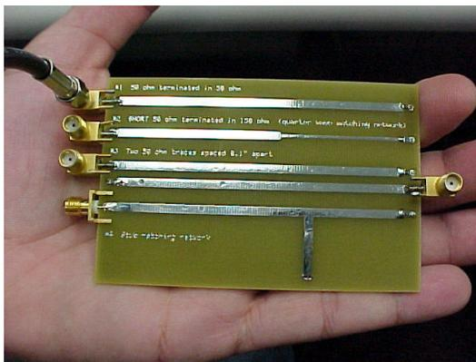
Figure 1 – Construction of a simple microstrip printed circuit.
