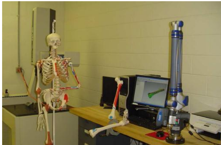
Figure 12. Scanning femur, patella, and tibia bone segments with a FARO arm
