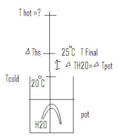
We are looking for the initial temperature of the Hot iron horseshoe before it was dropped in the water. We can find the initial temperature by looking for the temperature change between the hot horseshoe and the equilibrium temperature of the pot, water, and horseshoe. The change in temperature for water and pot is  $5^{\circ}$ C.
