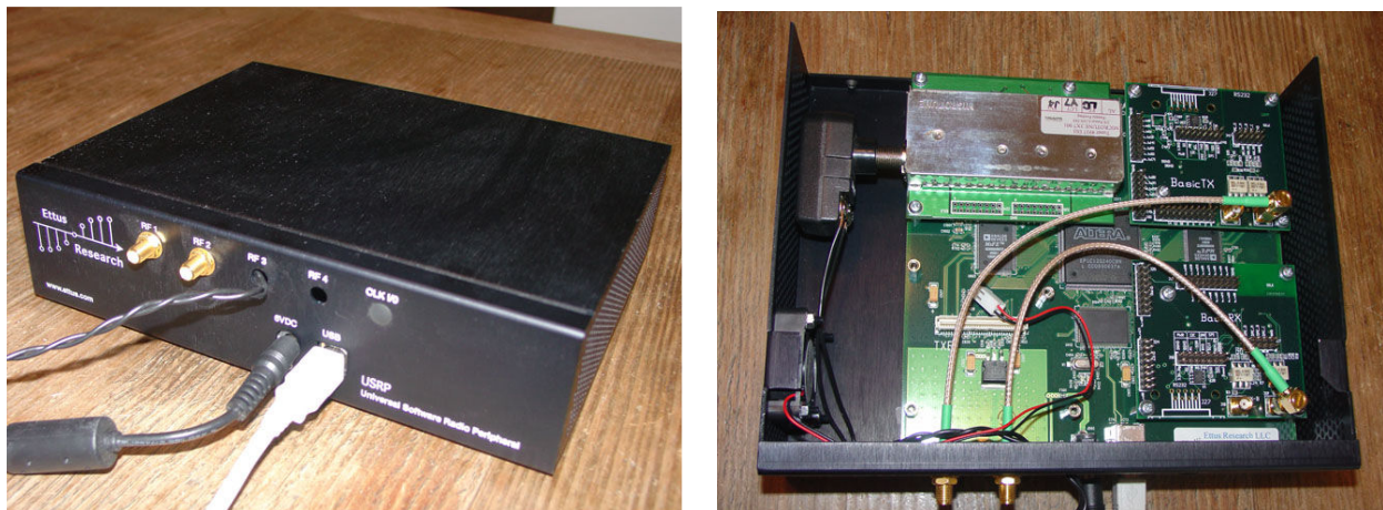
Figure 1. The USRP with the Cover On (left) and Off (right).
