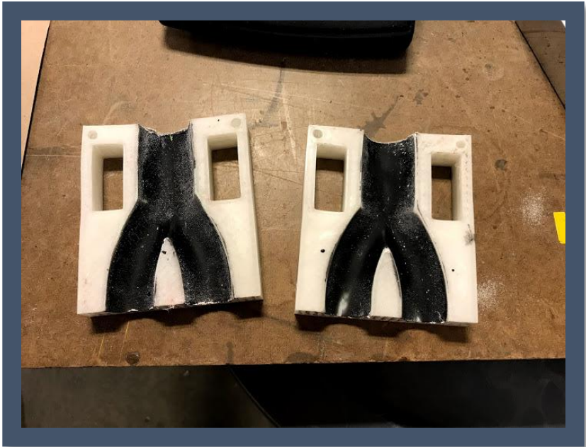
Soluble Ceramic Mandrel Mold
