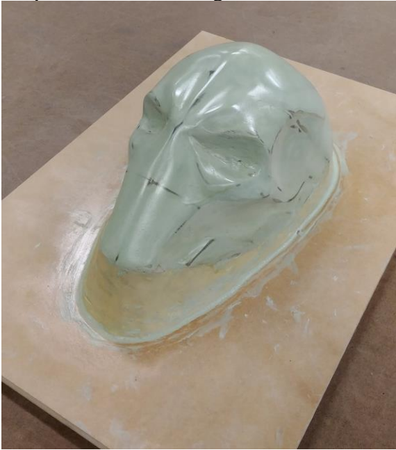
3D printed Male Tooling
