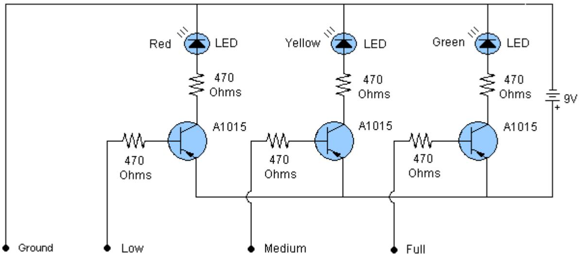
*Figure 2: Circuit diagram for water level indicator [Image].<sup>13</sup>*
