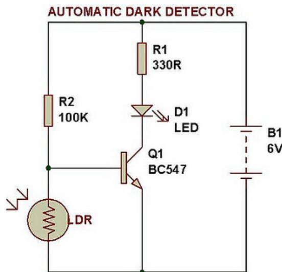
Figure 1: Automatic dark sensor circuit [Image].<sup>12</sup>
