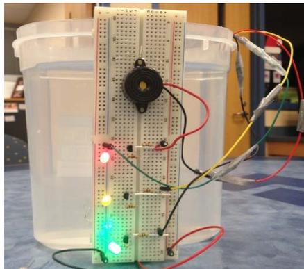
*Figure 3: Sensor developed to measure levels of water inside a tank. At level 3, which indicates the tank is full, the attached buzzer alarm goes off simultaneously as the red indicator light comes on*
