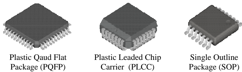
Fig. 1. Three common surface-mounting plastic packages 1
