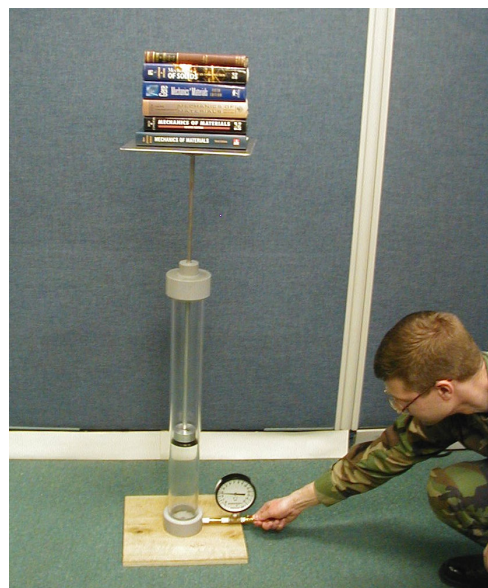
Figure 6: The Stress Demonstrator (on floor here, but best if on a desk) 18
