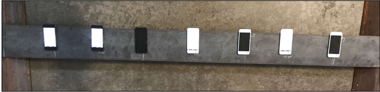
Figure 6. Simply supported prismatic steel beam with iPods placed for vibration measurement.
