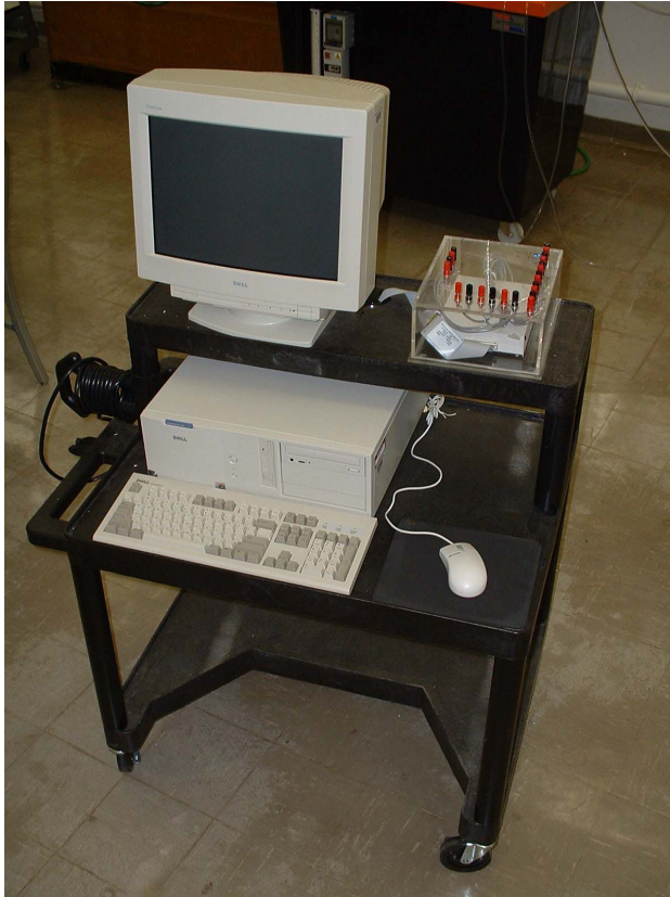
Figure 1. Rolling-Cart DAQ System used for Laboratory Monitoring and Control
