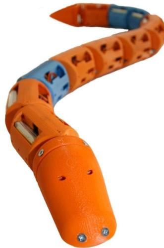
Figure 1: Robotic research platform for locomotion through granular media
