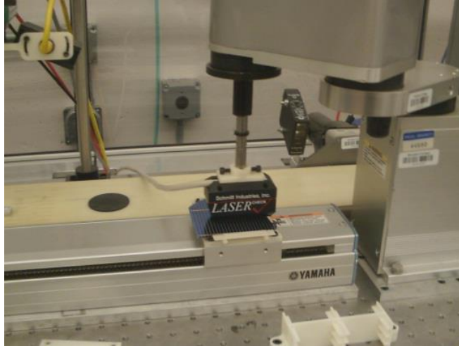
Figure 9: Robotic workcell for solar cell surface roughness measurement
