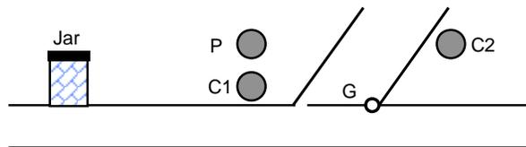
If a jar without a lid is detected, the controller activates a gate (G) that diverts the lidless jar off the conveyor to a defect area. Photocell C2 signals that the defective jar has cleared the exit conveyor. No jar will activate C1 and C2 at the same time.
