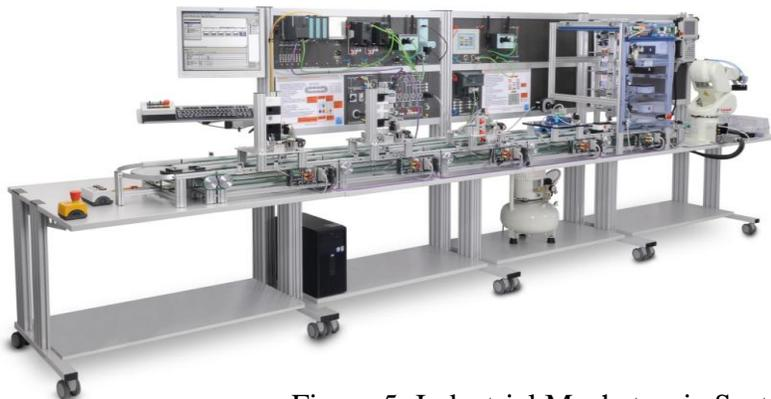
Figure 5: Industrial Mechatronic System From LN Company
