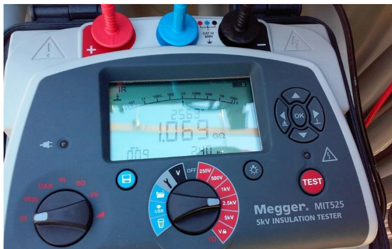
Figure 11. Insulation Resistance Tester Used for Testing
