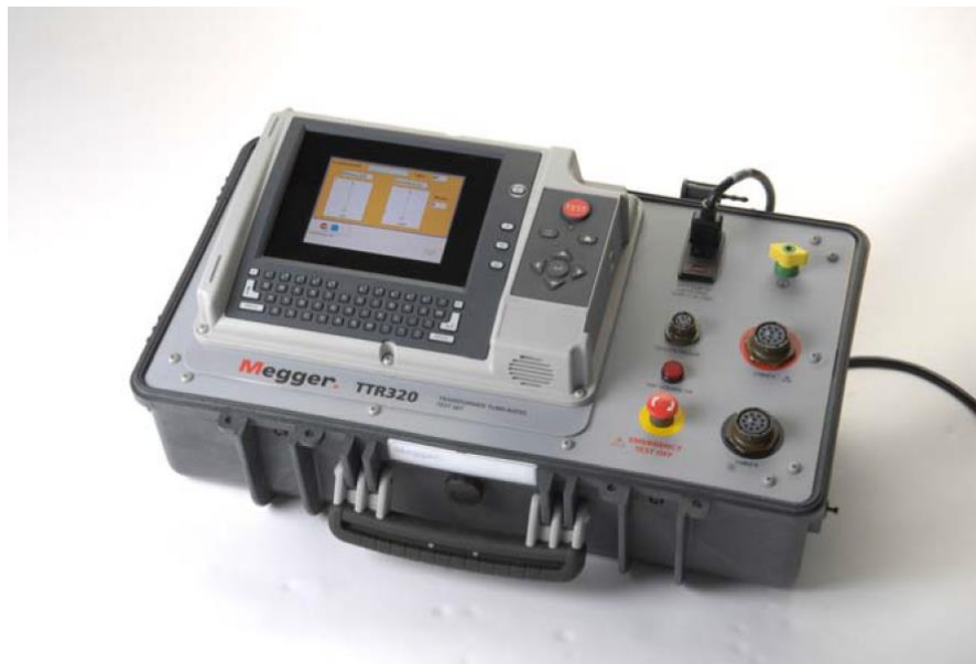
Figure 8. Megger TTR320 Turns Ratio Tester [From Megger TTR 320 User's Guide]
