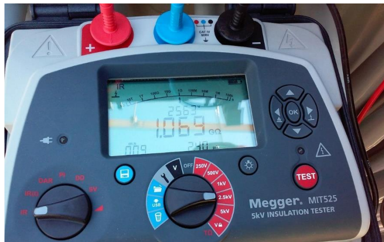
Figure 3. Insulation Resistance Tester Used for Testing
