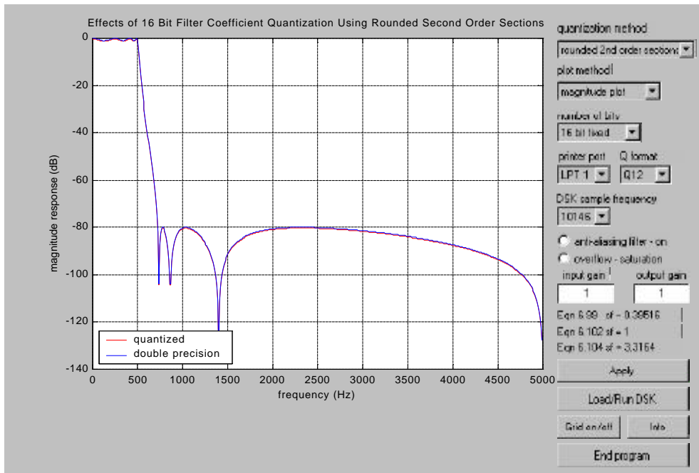
Figure 5. Magnitude plot of 7th order IIR Elliptic digital filter, quantized to 16 bits and implemented as a Direct Form II transpose using fixed-point algorithms.
