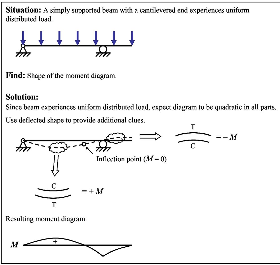
Figure 2. Example used in class to demonstrate how intuition about deflected shape helps one anticipate features of the moment diagram.
