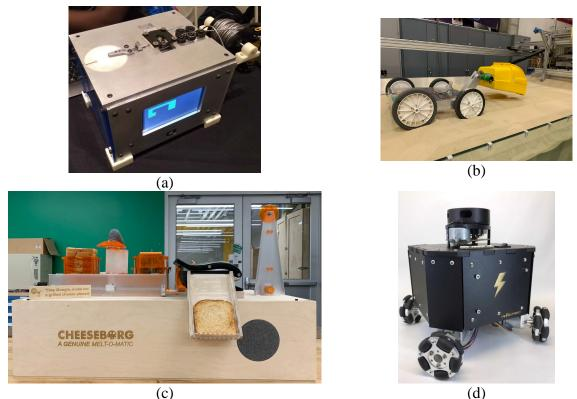
Figure 1: Sample student projects. Students explored a wide variety of concepts, including a CNC wire bender (a), a robot for beach cleanup (b), an automated grilled cheese maker (c), and a mobile drawing robot (d).
