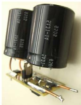
Figure 1. Energy transfer circuit used for Experiment #1
