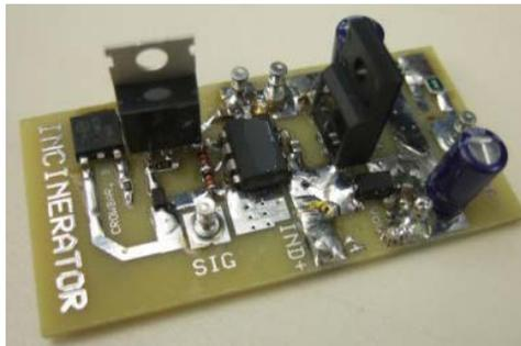
Figure 3. Buck converter test circuit for Experiment #3
