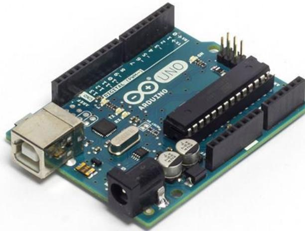
Figure 1 – Microcontroller Platform – Arduino Uno
