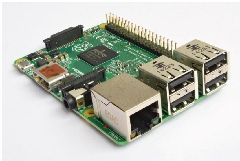
Figure 2 – Microprocessor Platform – Raspberry Pi 2 Model B
