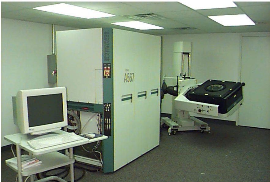
Figure 3 –The Teradyne Advanced Mixed Signal Tester. This instrument allows the students to program an automated sequence of tests to be performed by the tester. Components to be tested include voltage regulators to advanced mixed-signal chips such as DACs and ADCs.
