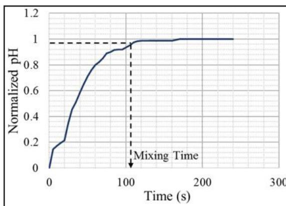
Figure 1. Typical plot of normalized pH vs. Time.
