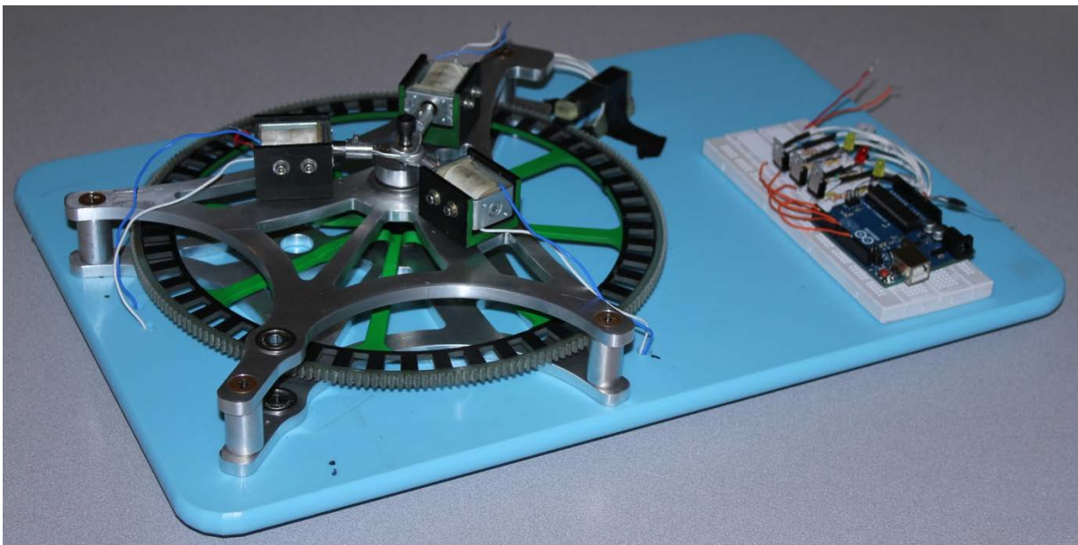
Figure 6: Engine from team in 3 rd place. Maximum Speed: 634 rpm; Kinetic Energy: 1.88 J; Speed-to-Mass Ratio: 215 rpm/kg
