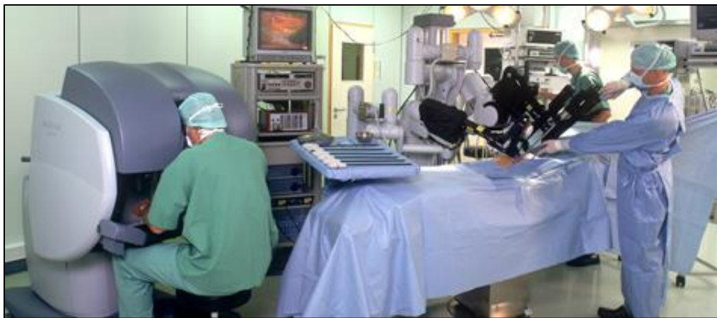
Figure 1. A typical operation room set up during robot assisted cardiac surgery. The surgeon (left) controls the robotic arms (middle) that operate on the patient. The surgeon's assistants (right) often help the surgeon perform the operation on the patient.
