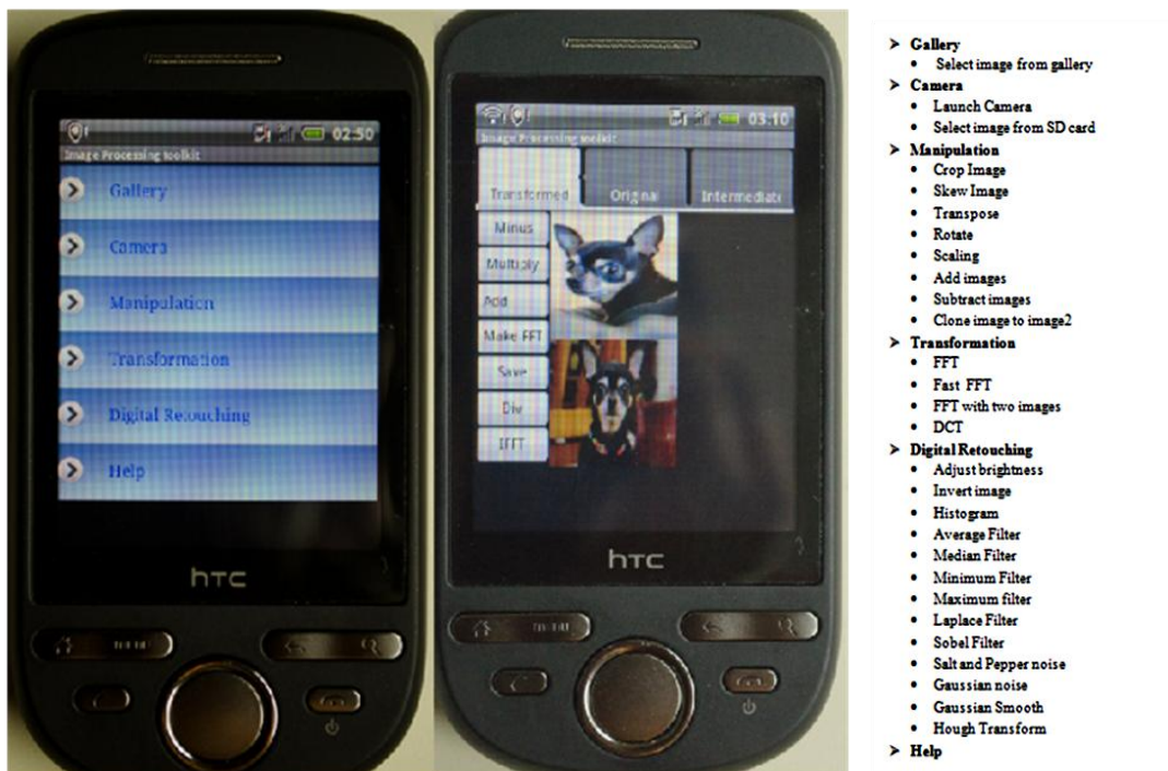
Figure 2. Menu structure display on Android phone(left hand side). On right side is the full ‘Menu’ structure implemented in this toolkit
