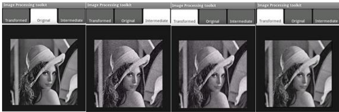
Figure 10. a) Original image; b) Gaussian noise added; c) Resultant image of Gaussian filter; d) resultant image of “Mean” filter.
