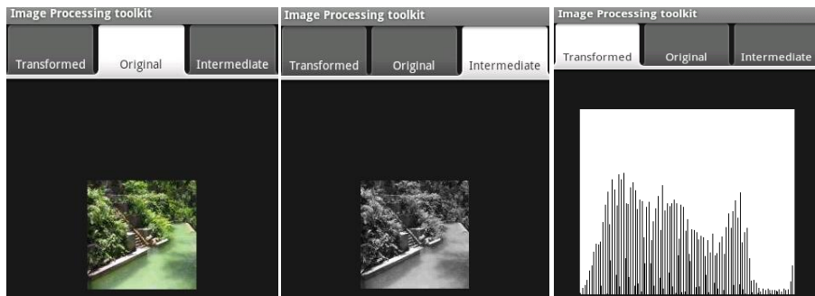
Figure 8 a) Original image; b) Grayscale image; c) Histogram
