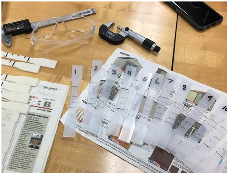
Figure 3 Clear cut-to-size LDPE specimens with measuring instruments and visible cross sectional area measurement locations 1, 2, and 3
