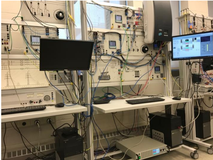
Fig. 1. Layout of residential microgrid for transactive energy experiments
