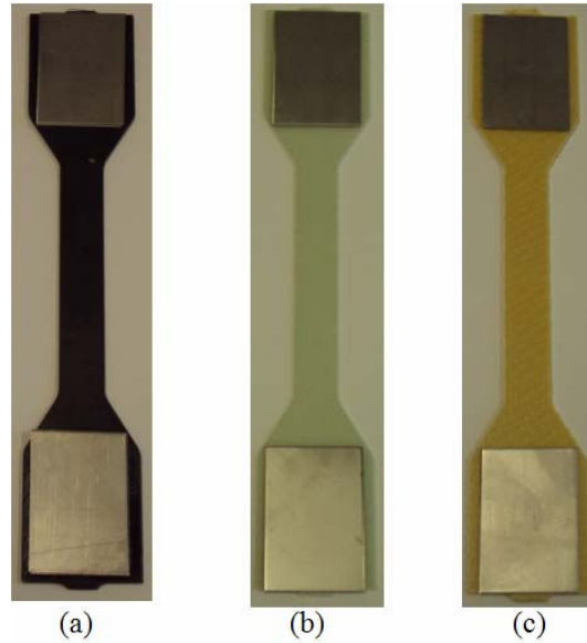
Figure 2: Composite samples used in tensile testing. (a) Carbon fiber, (b) Glass fiber, (c) Kevlar fiber
