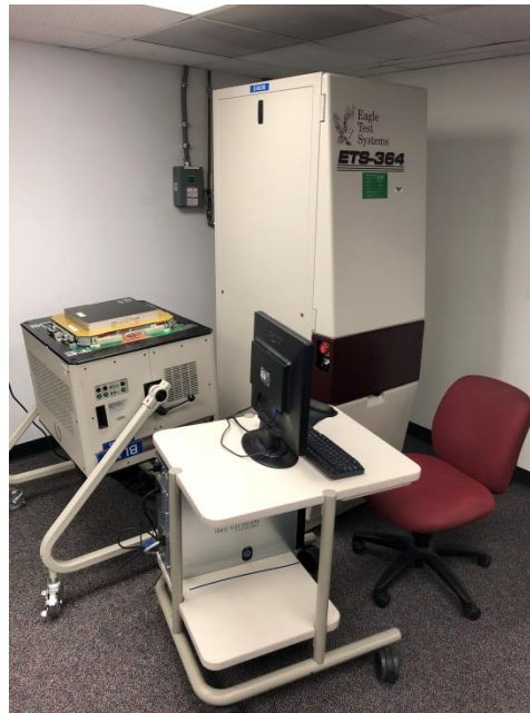
Figure 1. TI-supplied Teradyne Eagle ETS-364 production tester
