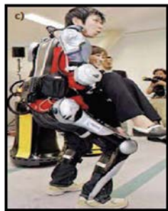
Figure 4: HAL, an exoskeleton system designed by the University of Tsukuba
