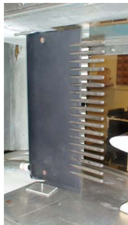
(a) Smoke Rake Assembly
