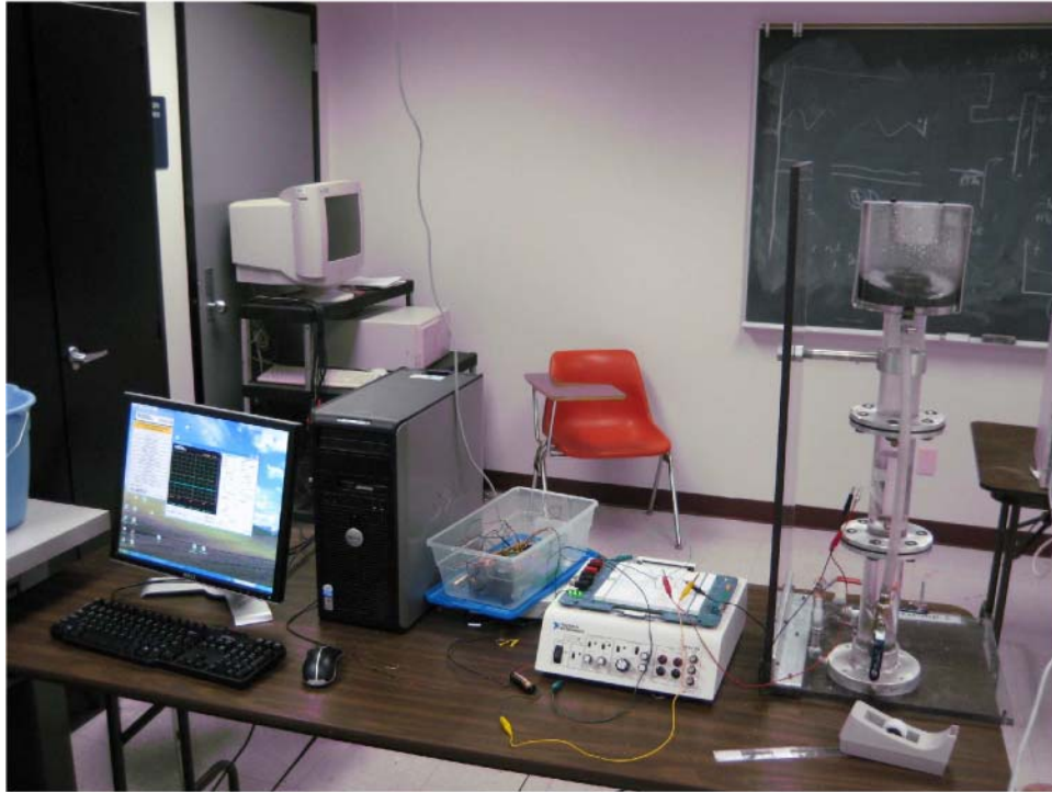
Figure 2: Experimental Station. Custom Made Statistical Column for Experimental Apparatus (right), ELVIS Virtual Instrument Suite and the Benchtop Workstation with Prototyping Board (in the middle), and Computer-Aided Data Acquisition System (CADAS) (left).
