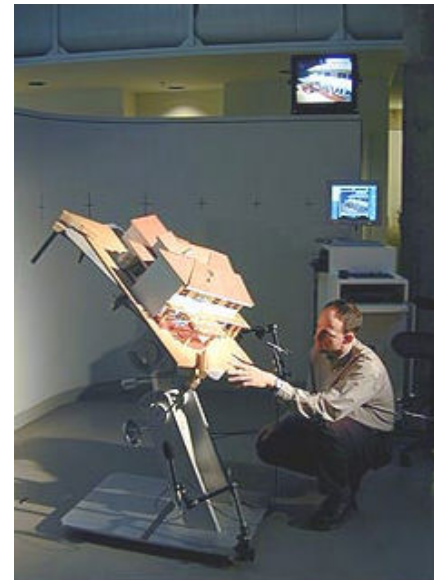
Figure 4: Tilting Table Heliodon
