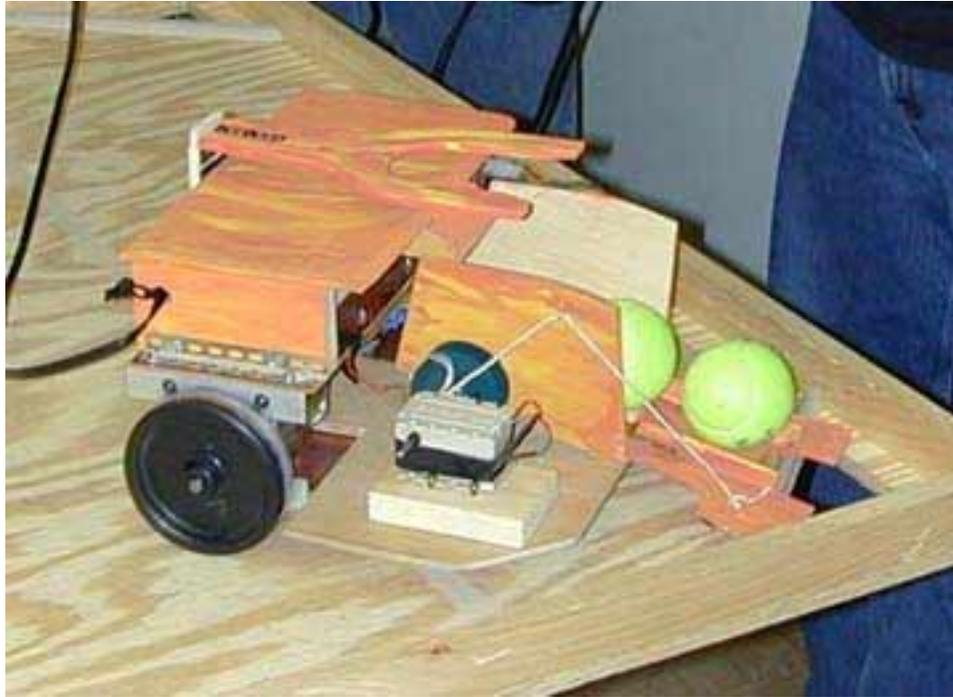
Figure 4. Unloading balls that were pushed into the carrier using the U-shaped arm
