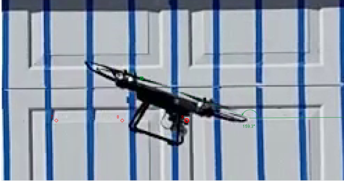
Figure 6. Screen capture from the video clip of a drone flying in front of a ruled background.
