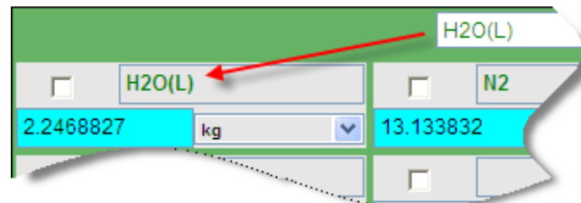
Figure 10. To obtain a higher heating value, de-select H2O and select H2O(L) from the products menu. Select Balance Reaction from the action menu and then press Super-Calculate to update all results.
