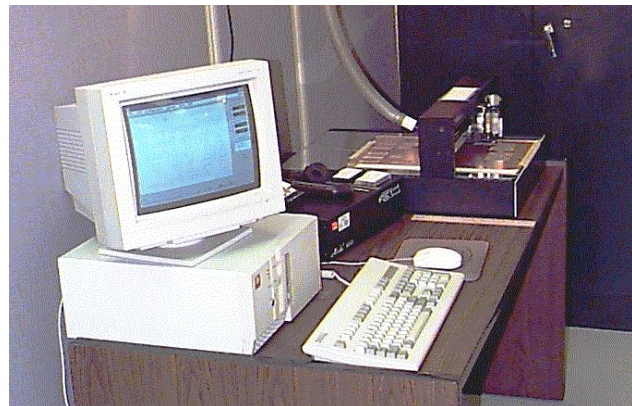
Figure 4. The dedicated computer and controller with the QC-7000 Mill/drill machine in the back.
