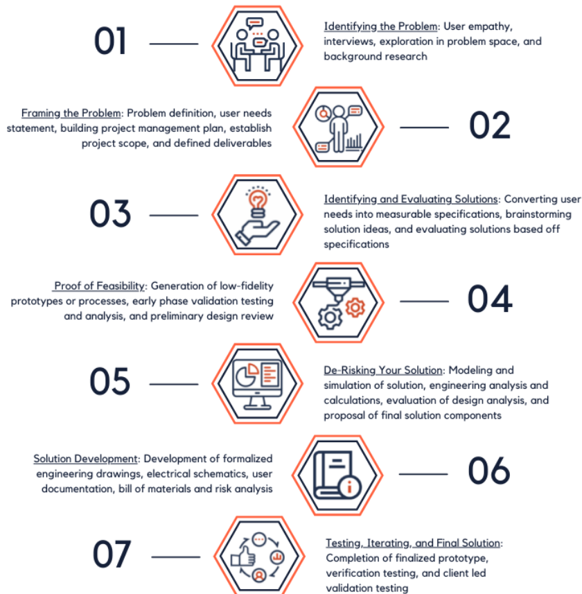
Figure 3. The design firm capstone studio model makes use of milestones or design phases to ensure students’ progress through all phases of the design process and meet course requirements
