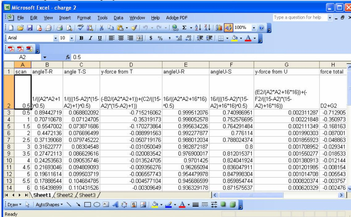
The above Excel columns are used to compute the vertical forces on the horizontal bar as exerted by the vertical bar. The vertical bar scan across the horizontal bar and a plot of force versus scan distance can be generated. A log-log plot would extract the power law dependence of force versus distance. The simulation result can be used to compare to the experimental data when the
