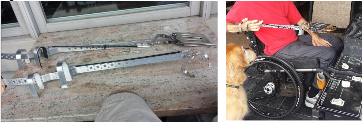
Figure 1. A prototype device for flipping burgers for use by a man with limited hand dexterity.
