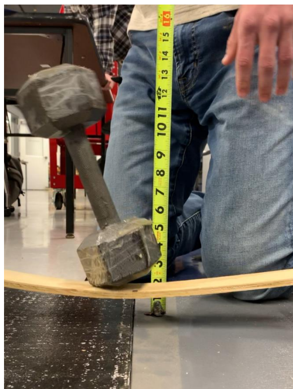
Figure 6 Loads applied to beam made of plywood
