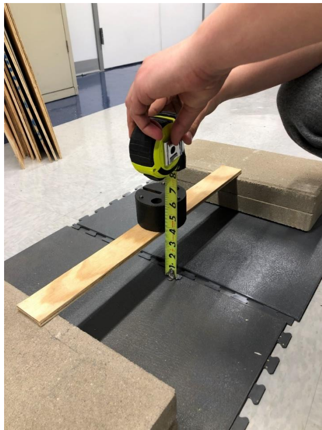
Figure 8 Measuring static deflection of a plywood beam
