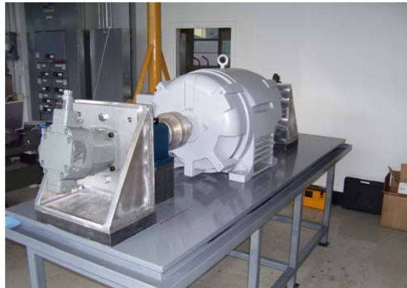
Figure 3 Current status of the hydraulic hybrid vehicle test stand.
