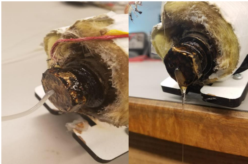
Figure 3: Left: Shows the extrusion of a 50-50 blend of PET and PETG mixture. Right: The extrusion of just the PET bottles. Notice the low viscosity and inability to create the desired filament.
