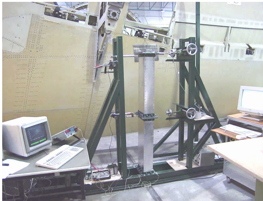
Figure 1: The result of the first year project: a satellite box in its test rig (photo courtesy of Ir. A.W.H. Klompé)
