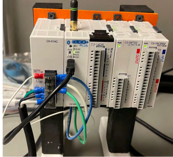
Figure 1: CLICK Plus PLC used in these lab experiences
