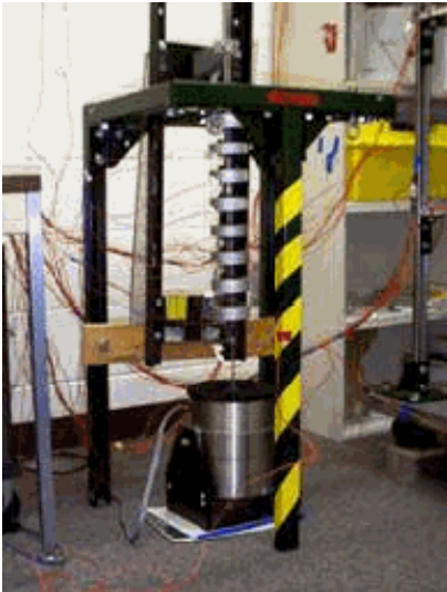
Figure 1. An 8-DOF system that can be modified by changing springs or putting bumpers between masses.
