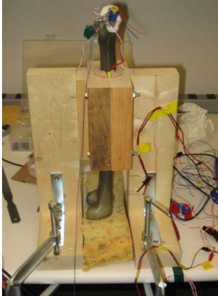
Figure 3. The test setup used for a project involving detecting when a hip prosthesis is fully seated in a simulated femur.
